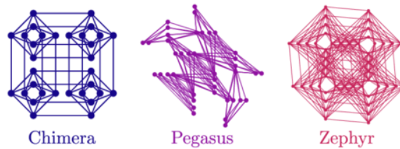
Figure 1: Schematic illustration three D-Wave topologies: Chimera, Pegasus, and Zephyr. In the Zephyr topology, each qubit is connected to up to 20 neighbors, enabling denser logical graph embeddings with shorter chains compared to earlier Chimera and Pegasus architectures [2].
