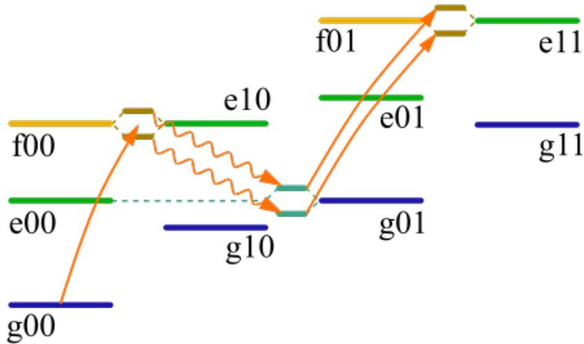
Figure 1: Energy levels of the transmon laser. The letter is transmon level, the first number is the number of photons in the auxiliary resonator, the second number — in the reservoir (e.g.  $g_{10}$  means that there is 1 photon in the auxiliary resonator and 0 — in the reservoir)
